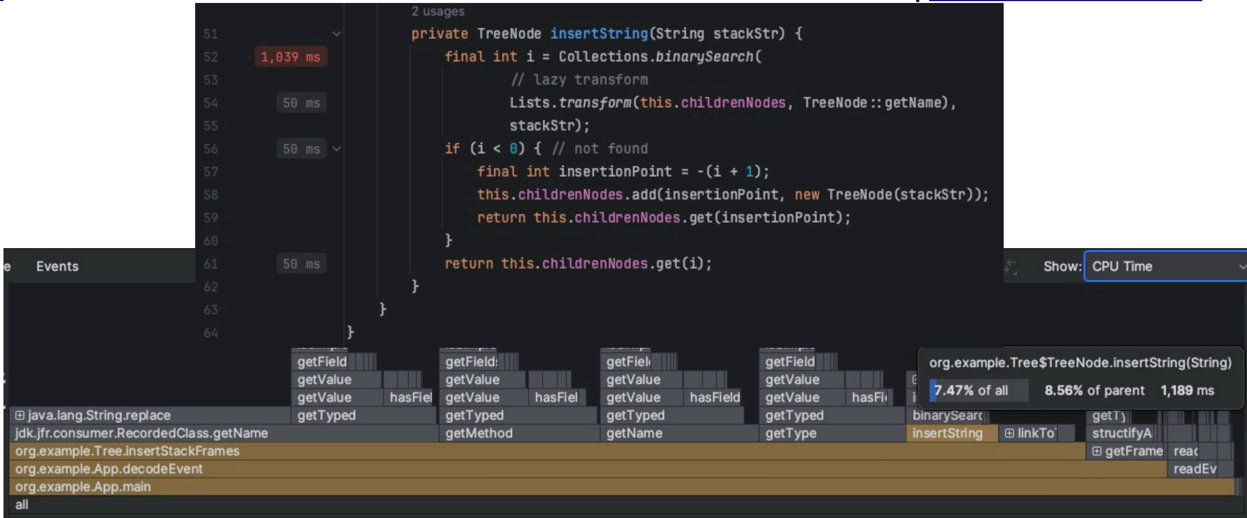
FIG. Another performance issue: too many binary searches during insertion even if binary search has O(\log N) complexity
