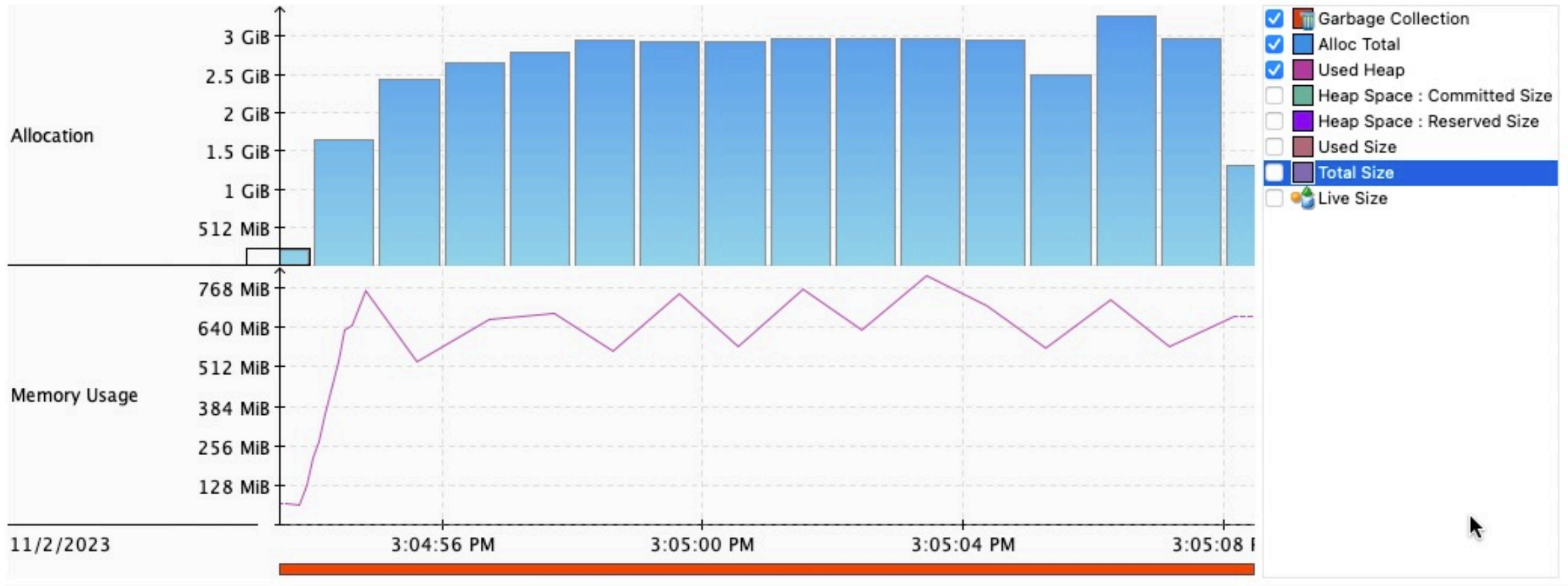
FIG. Memory issue: large heap size while building the call stack with millions of (allocation) events
